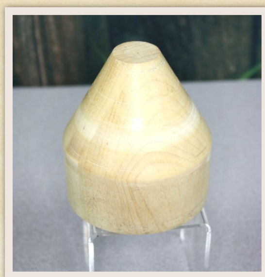
Left: Two Maple goblets. Right: Custom made tail stock support for the goblets.
