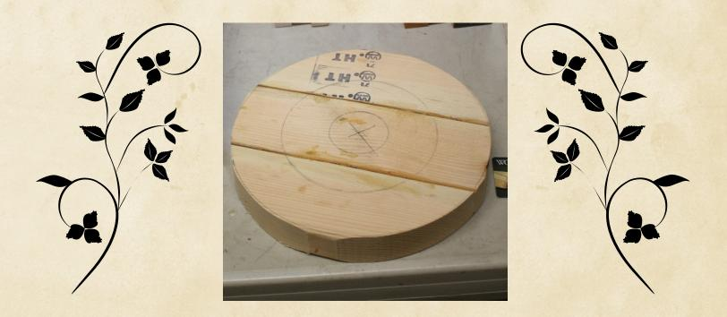
He decided to demonstrate turning a plate. To show how to keep your costs down, Sid used a 2 X 4. He jointed the sides, cut them to length and glued the edges together. After the glue dried, he marked his center. He then cut a disk (shown above) on the band saw. He made several disks at the same time.
